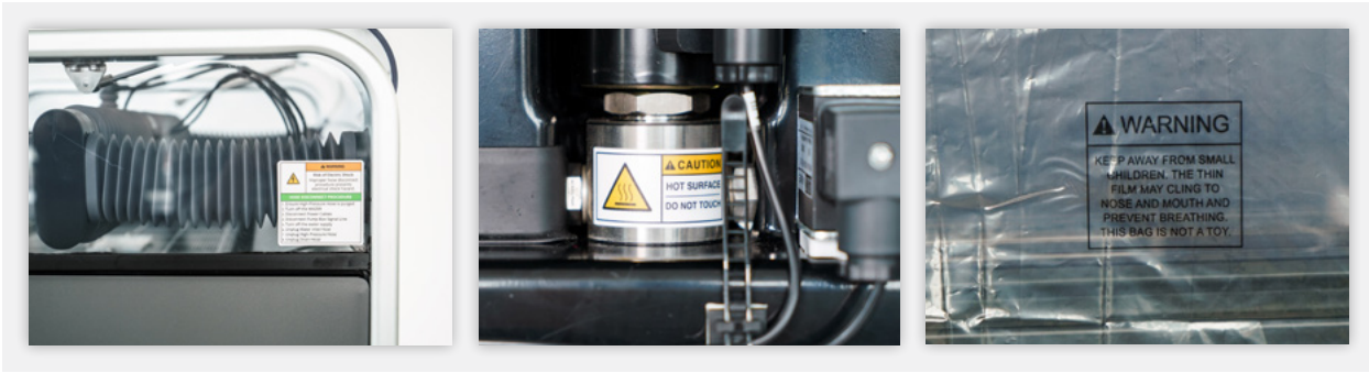
This label warns you of the electric shock hazard associated with an improper hose disconnect procedure. It also serves to instruct you of the proper disconnect procedure.
